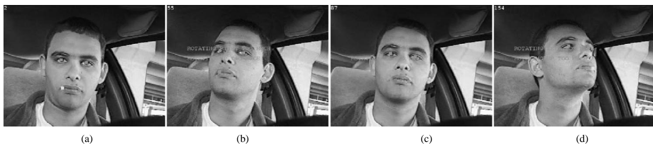
Fig. 19. Driver visual attention output. (a) No messages, (b) rotating right too much, (c) no messages, and (d) rotating left and up too much.
