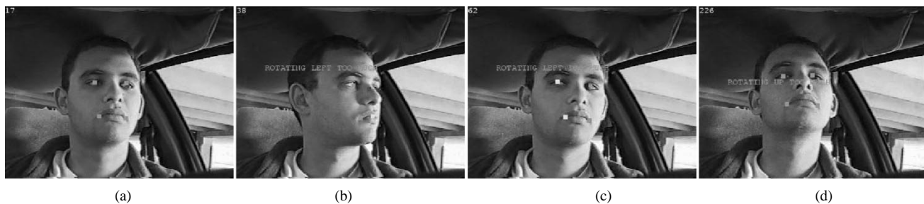
Fig. 18. Driver visual attention output. (a) No messages, (b) rotating left too much, (c) rotating left too much, and (d) rotating up too much.
