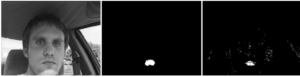
Fig. 1. Lip color predicate training. The first image is the original image, the second shows the manually selected skin color regions, and the third shows automatically detected lip regions.
