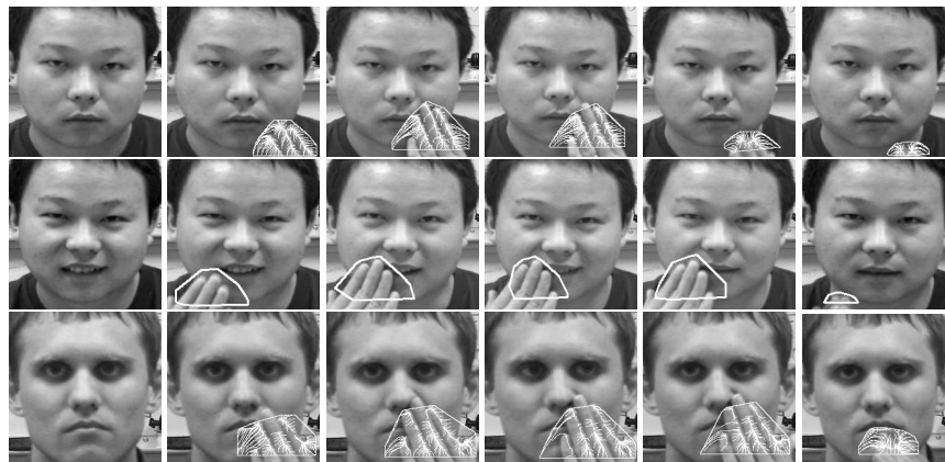
Fig. 6. Hand segmentation results for three sequences. Row 1 shows channel lines superimposed. Row 2 shows the convex hull. The sequence in Row 3 involves occlusion for over 300 frames.
