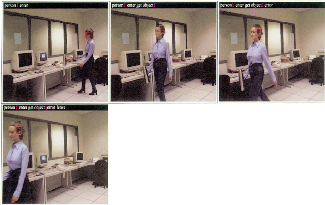
Fig. 9. A Person enters the room, picks up a thermos, but the tracking algorithm loses the thermos so an error is output, finally the person leaves the room (170 frames, 4 key frames).
