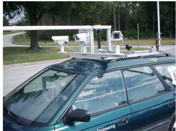
Figure 2: Our experimental UGV is a Subaru Outback with an autopilot system and three cameras mounted to the roof.
