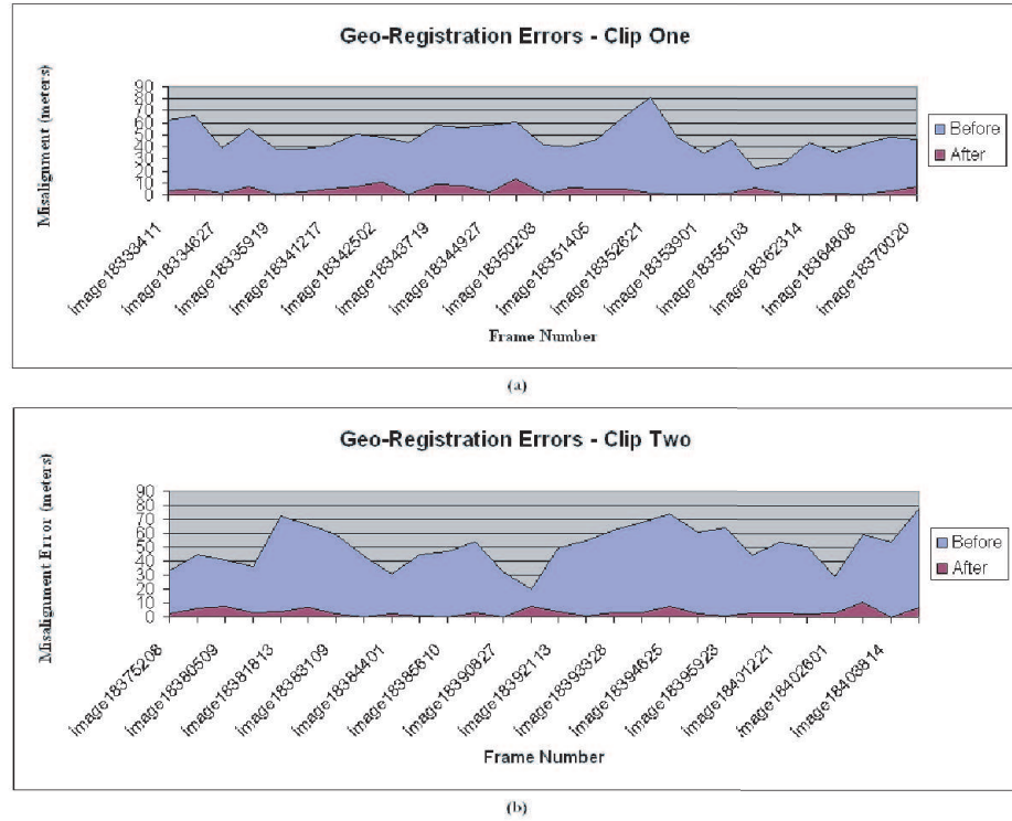
Figure 7.12. Misalignment errors. (a) Clip One: The pre-alignment and post-alignment errors for 30 frames. A pre-registration average error of 47.68 meters with a standard deviation of 12.47 and a post-registration average error of 4.34 meters and standard deviation of 3.19 per frame was recorded. (b) Clip Two: The pre-alignment and post-alignment errors for 30 frames. A pre-registration error of 51.43 meters with a standard deviation of 14.66 and a post-registration average error of 3.46 and a standard deviation of 2.91 was recorded.
