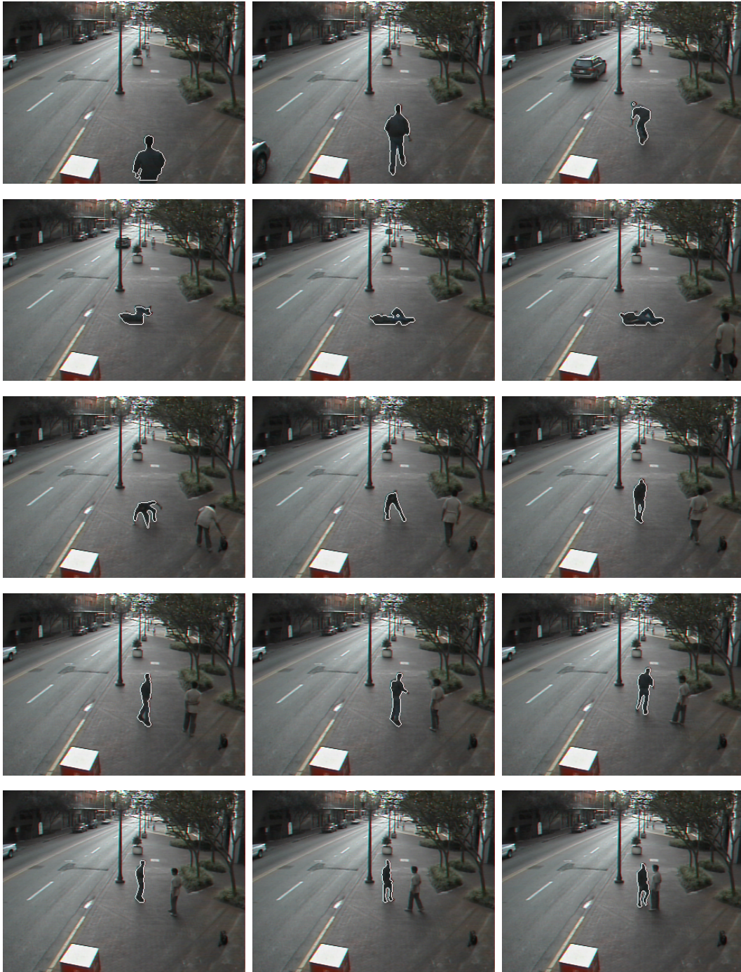
Figure 5.13: Contour tracking results for a sequence acquired from a stationary surveillance camera.
