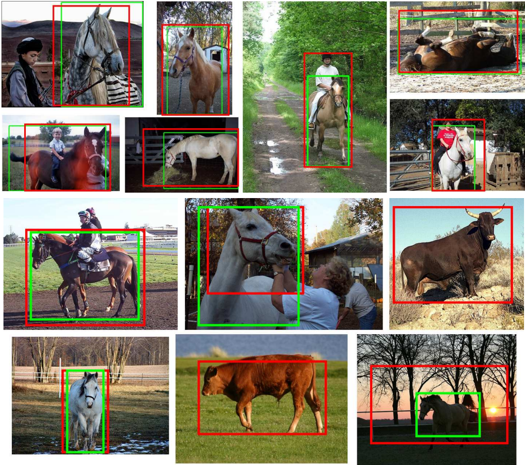
Figure 6.5: Detection of horses in the PASCAL VOC dataset using our approach. The ground truth is shown in green and red boxes display our detected results.
