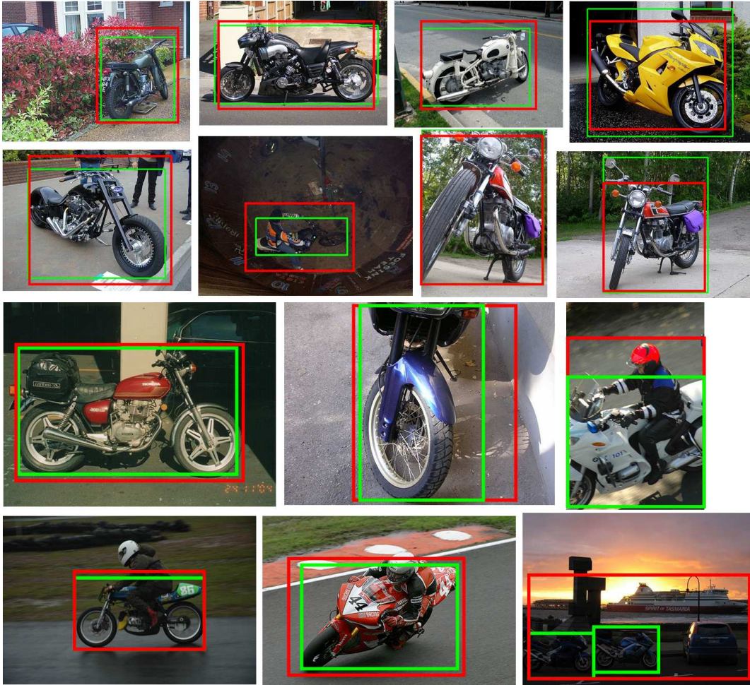
Figure 6.4: Detection of motorbikes in the PASCAL VOC dataset using our approach. The ground truth is shown in green and red boxes display our detected results.
