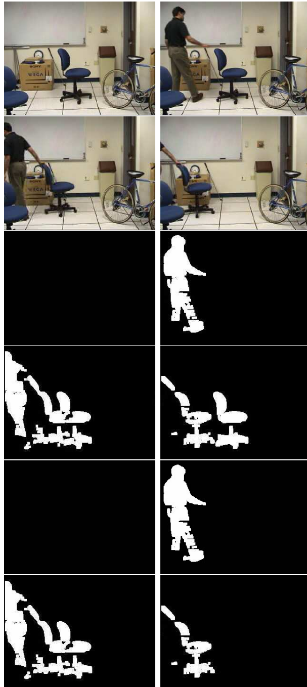
Figure 2.5: Removal of a static (background) object from the scene. The first two rows show images at an interval of 30 frames from a sequence. The 3rd and the 4th row show the color based results using the mixture of Gaussians. The last two rows show the hierarchical background subtraction results. Note that the removal of object is successfully detected and the uncovered area does not show up as foreground region.
