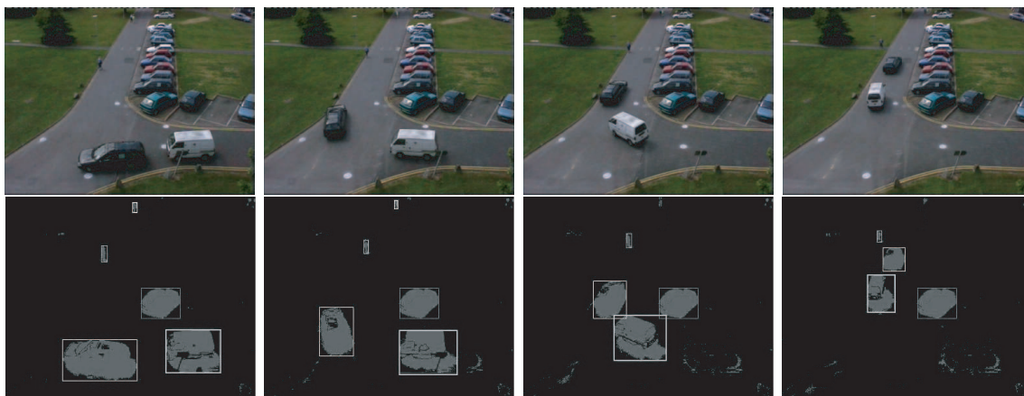
Figure 4.1: PETS Dataset 1, test, camera 2 sequence (frames 2440-2580). The first row shows the images. The second row shows regions obtained by background subtraction along with their bounding boxes
