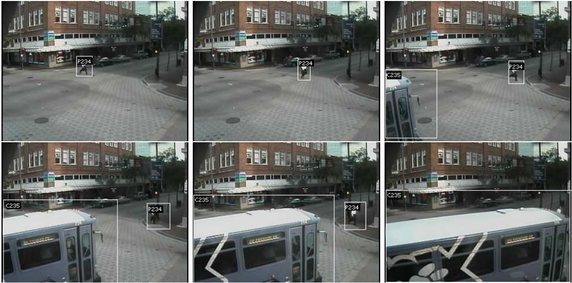
Figure 4.6: Orlando down town. A person being completely occluded by a bus. Since the position plus predicted velocity of the person is near the frame boundary, the person is determined to have exit the frame.
