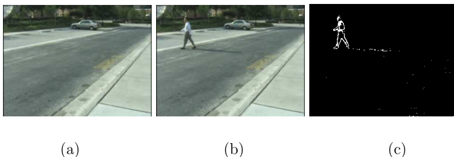
Figure 2.1: Gradient based subtraction results, (a) first image in the sequence (b)150th image (c) gradient based subtraction. There is some noise but it can easily be removed by size based filtering.
