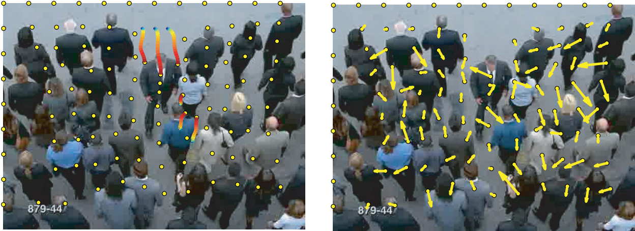
Figure 3.3: An example of particle advection using the average optical flow field and the corresponding interaction forces. (Left) The trajectories of a small set of particles are depicted for demonstration. (Right) The set of computed interaction forces of particles.
