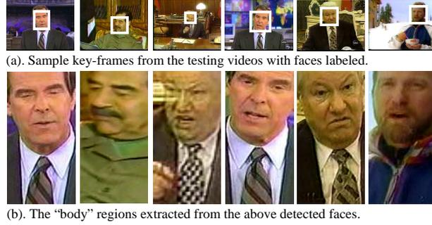
**Figure 4.1:** (a). The sample key frames with the detected faces; (b). The body regions extended from the faces. Global feature comparison or face correlation fails to link the same person in these examples, while the comparison of the "body" regions provides the meaningful information.
