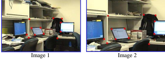
Figure 7: Two images from a zooming sequences. The red points represent the correspondences in the images. The scaling factor \lambda \approx 1.55 , and the principle point is [177.9, 116.0] , which is very close to the image center (image size is [360] \times [240] ).
