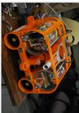
◆ The AUV has two cameras — a forward camera and a floor camera.
